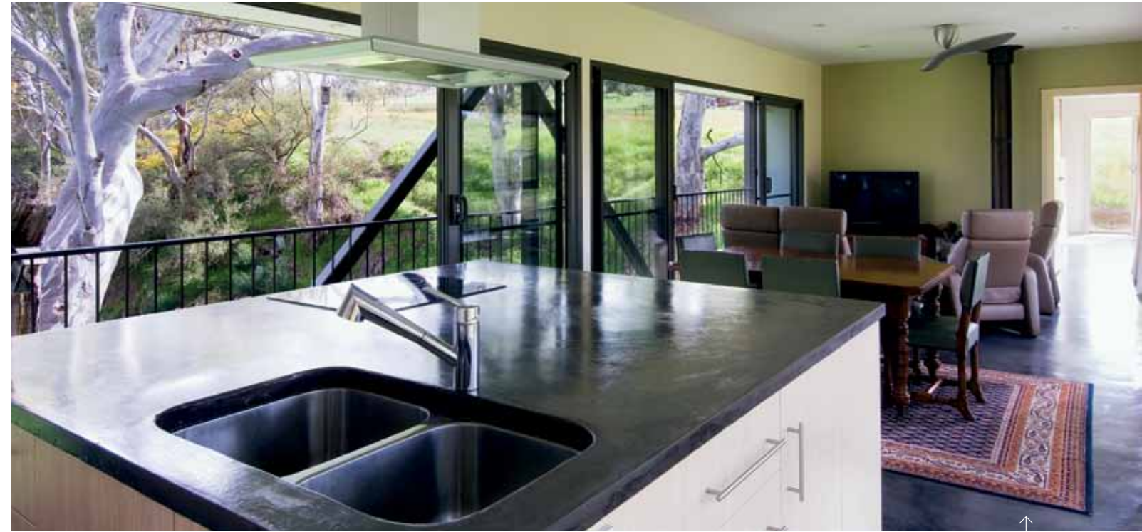
↑ The dark colour rendering of the concrete slab encourages heat absorption during winter
