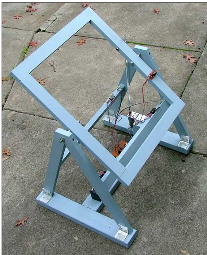
The solar tracker test frame used to develop the tracker controller.
