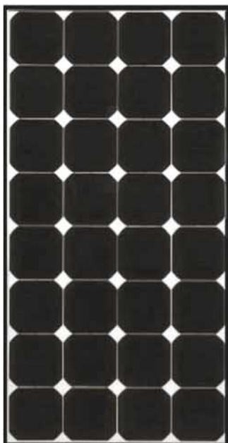
SPR-95, 95W 1038mm x 527mm 17.4% module efficiency
