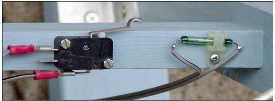
The limit switches. The primary reed switch is on the right, the 10 amp secondary microswitch is on the left. The reed switch is triggered by a small magnet attached to the moving array frame.
