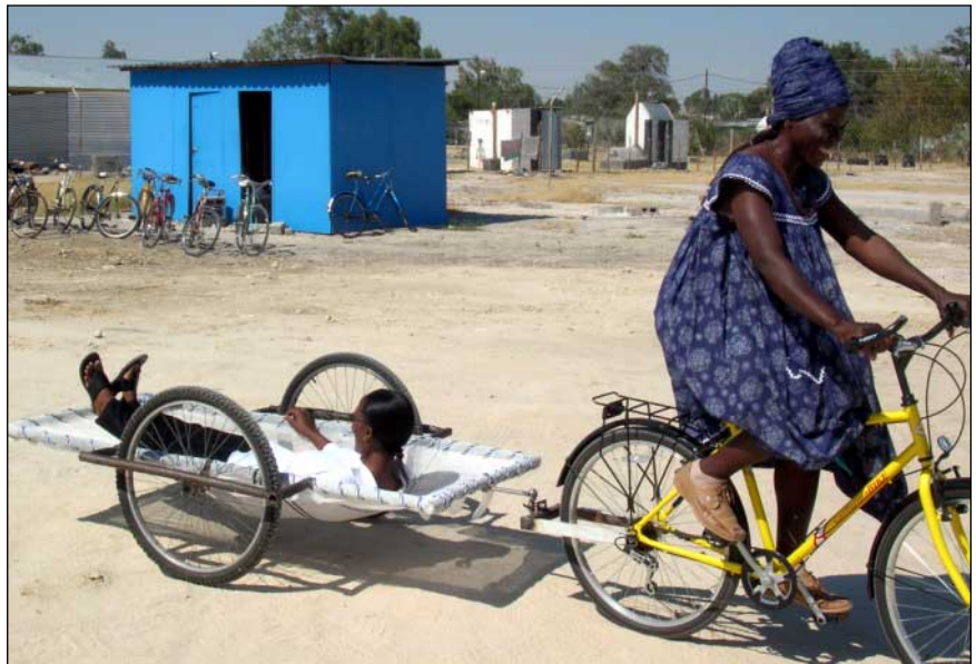
Top: Mr Elephant inside his bike shop. Bottom: HIV/AIDS home based carer Meme Gudrun tests a prototype bicycle ambulance developed by BEN Namibia for emergency medical transport.
