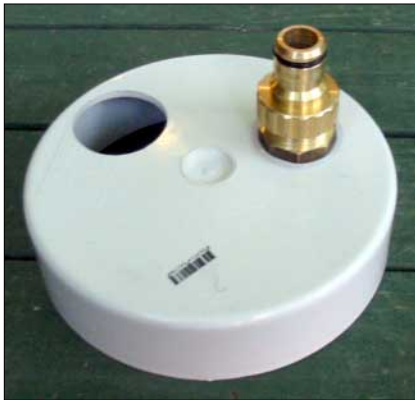
The lower end cap has two holes cut into it. One is fitted with a hose connection, while the overflow pipe is glued into the other.
