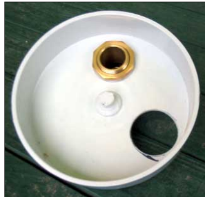
The lower end cap has two holes cut into it. One is fitted with a hose connection, while the overflow pipe is glued into the other.
