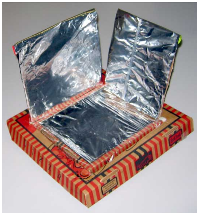
A simple solar cooker made from a couple of pizza boxes!
