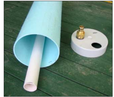
The overflow pipe is placed inside the diverter, the bottom end cap is slipped over it, and the two are glued together.
