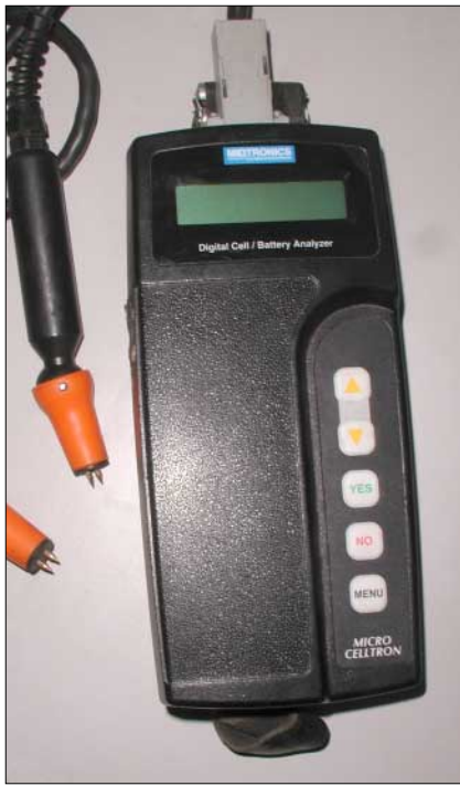
The Celltron CTM-100 conductance analyser used in the study. The battery test probes have two spring-loaded pins which dig into the lead terminal posts. This is called a ‘Kelvin’ connection, and allows the instrument to measure currents and voltages at the point of connection with the battery posts.
