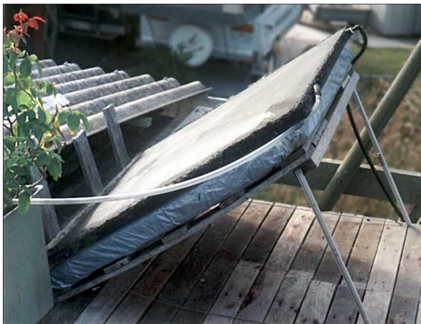
The completed solar collector on its simple stand.
