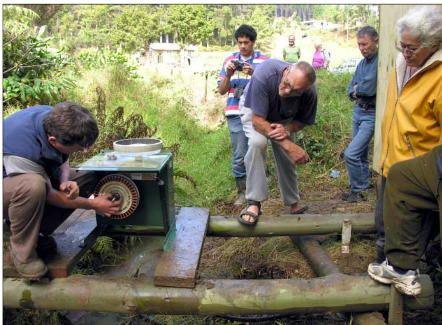
Adjusting the speed for maximum efficiency.
