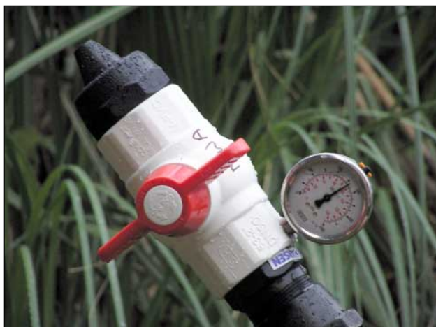
Left: The turbine is tested and protected from damaging UV rays. Right: Jet and pressure gauge is mounted on the line .
