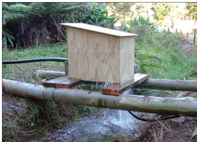
Left: The turbine is tested and protected from damaging UV rays. Right: Jet and pressure gauge is mounted on the line .
