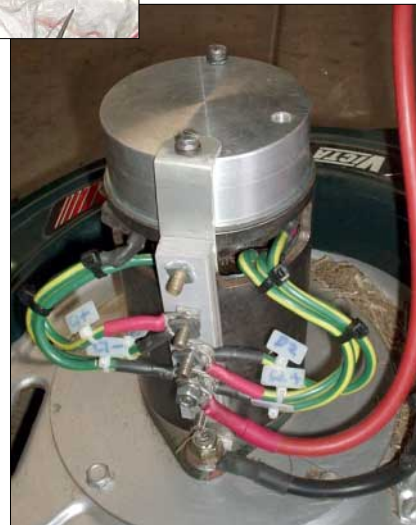
Bruce rebuilt the motor to suit the mower. Above you can see the reworked armature, while at right is the completed motor and new top bearing mount.
