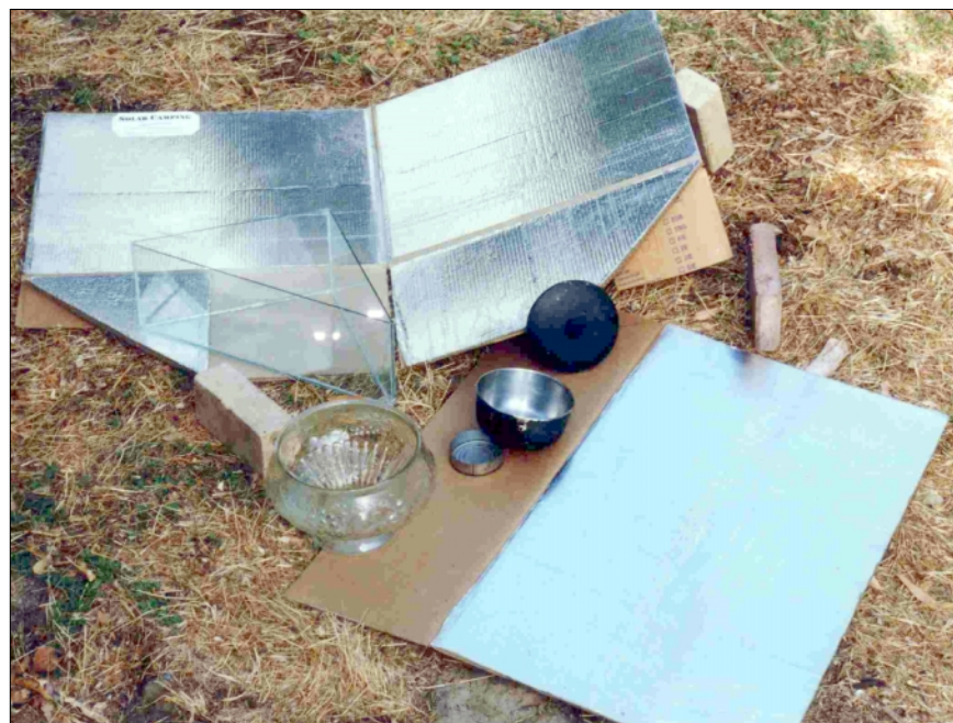
The parts of the cooker made by the SAS workshop participant. All the cardboard parts can be carried flat and fitted together in the field.
