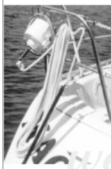
Aquair U.W. A submerged water powered generator with rate of 8 Amps for 12/24 volt charging.
