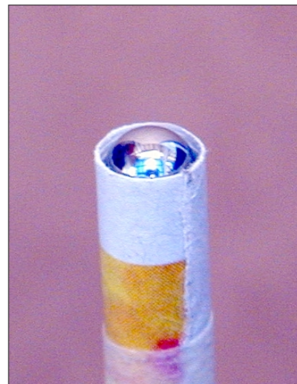
This is the end of the dowel used to form the foil jitterbug casing. See how the ball bearing sticks out above the paper sleeve.
