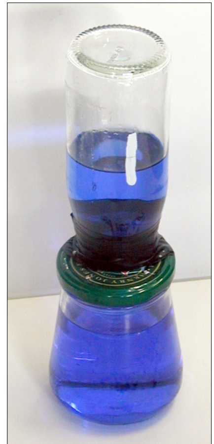
A jar, a bottle and some coloured water is all you need to measure the pressure of the Earth's atmosphere. A bottle with a thinner, longer neck would be better than the one used here.
