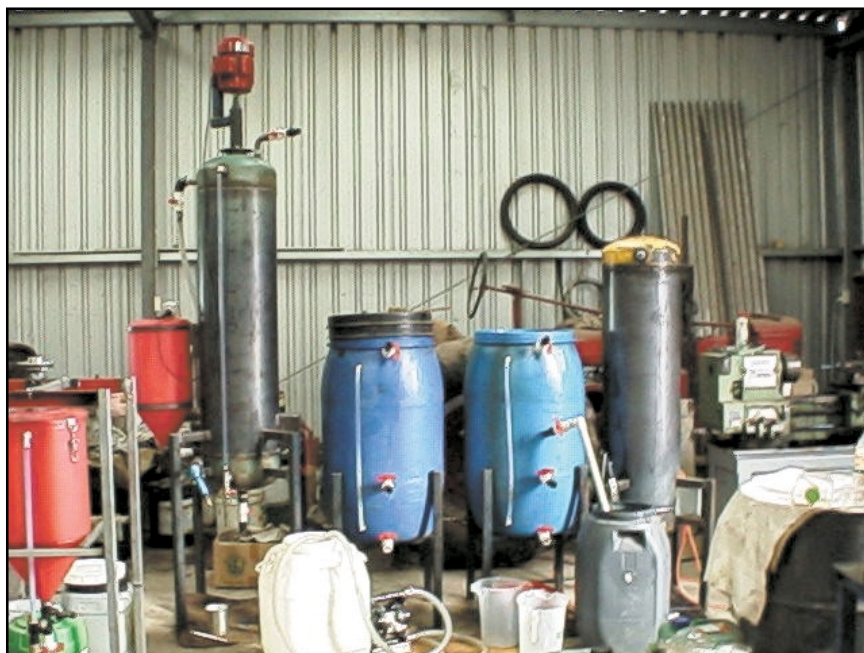
Steven Hobbs' mini biodiesel plant in the shed at his farm.
