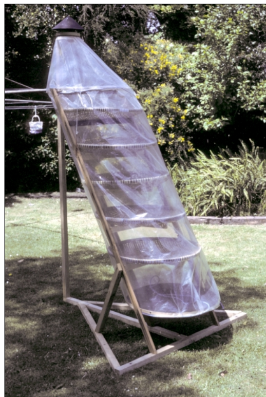
A bamboo tray solar dryer.
