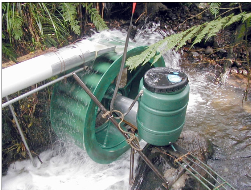
Power generation from a simple waterwheel is possible using a washing machine motor!
