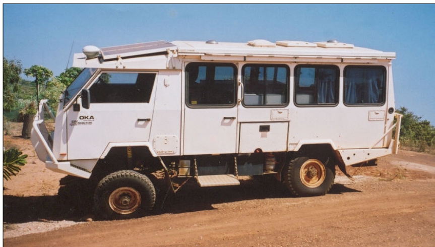
The front axle has neither broken nor is falling off! Illustrating the huge axle movement of these vehicles, the opposite front wheel is on a rock over 1200 mm high.
