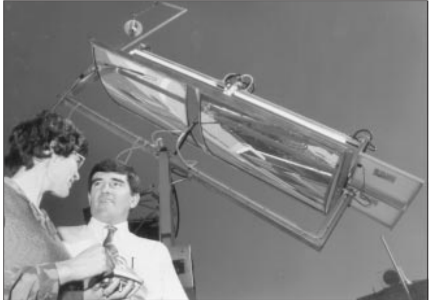
Solahart have won a federal government grant to research concentrating troughs for electricity generation. The troughs focus the sun's energy on special photovoltaic panels. Solahart technical manager, Mal Hayes, is pictured with Dr Adele Milne, the project manager from industry partner, Western Power.
