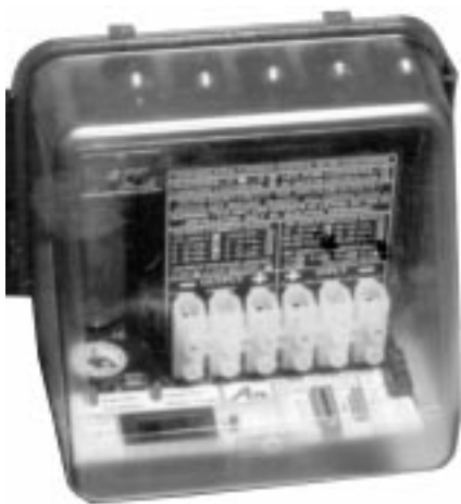
The maximiser from AERL will actually boost the current going into the batteries.
