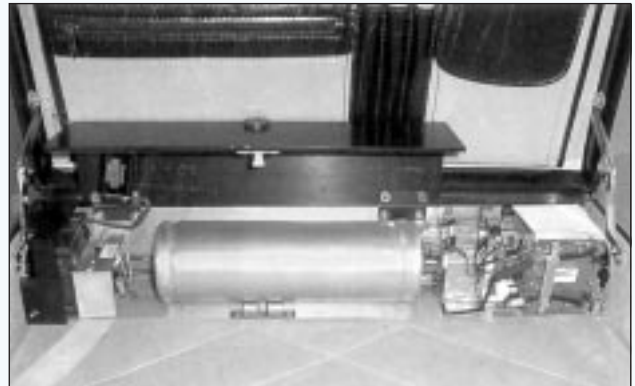
The fuel cell system is so small it can be mounted inside a briefcase for powering a laptop computer.
