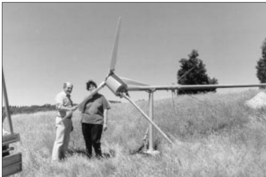
Above: Linda White and friend with a turbine lowered for inspection. Note the rest for the tower to sit on when lowered.
