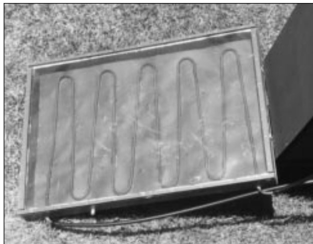
Here you can clearly see the serpentine shape of the copper pipe in the solar collector panel.
