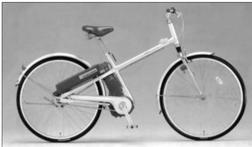
The state of the art is illustrated by the jointly developed Yamaha/Bridgestone 'cross framed' bicycle with aluminium parts and 26" wheels with sprung front forks. This PAB weighs 26kg, will travel 28km on a single battery charge, has power output of 235 watts and is recharged in 3.5 hours from mains electricity.
