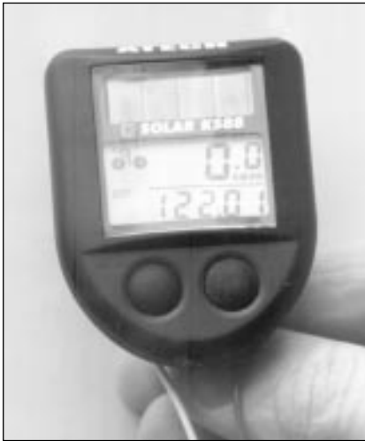
The bicycle computer used to record the wind data.
