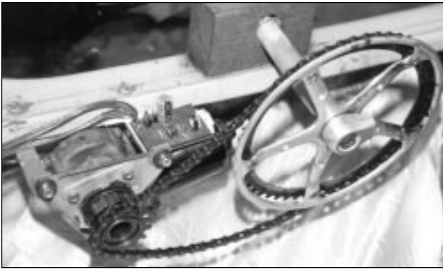
Here you can see a close-up of the motor and sprockets. Note the maximiser attached to the back of the motor with double-sided tape and glue.
