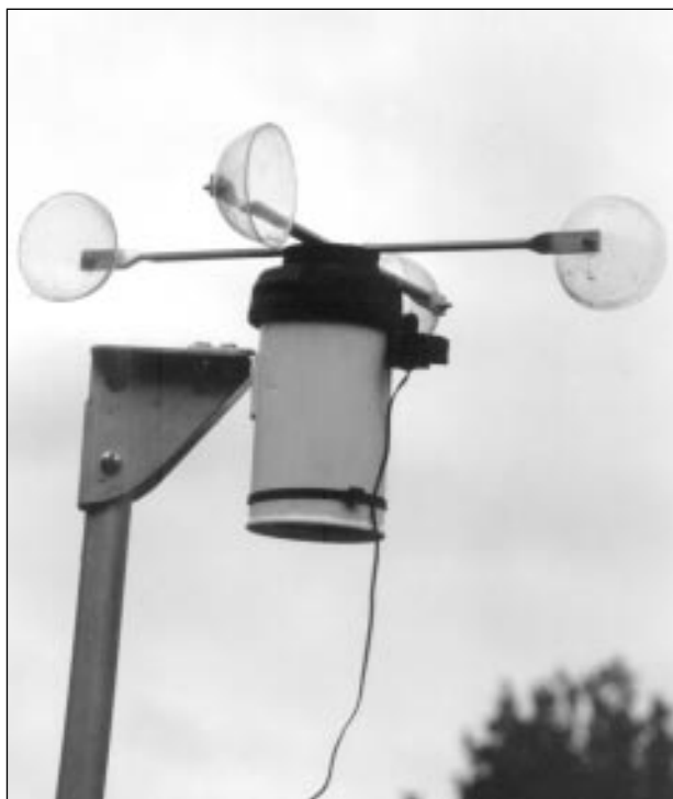
The anemometer section of the wind data logger is easy to build and costs just a few dollars.
