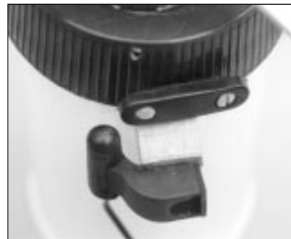
How the sensor is mounted on the side of the anemometer case.
