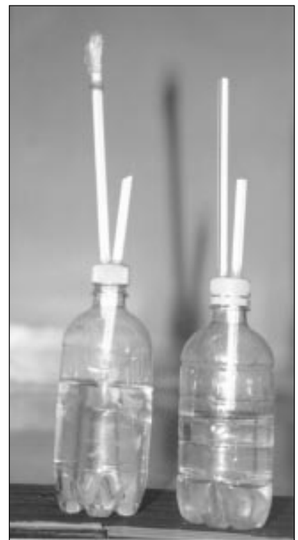
The syphon is on the right, while the pump is on the left.
