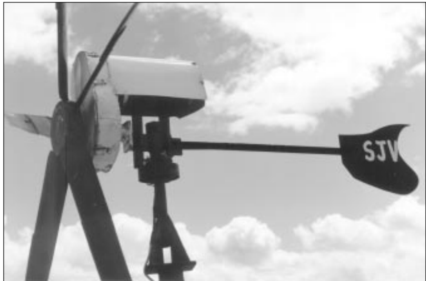
Sam's home-made wind generator produces power using an old DC motor.
