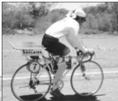
Bottom left: Pinocchio from Italy was one of the most striking entrants in the Cycle Challenge with its bamboo fairing. Left: Anyone for 3,000 km of desert? This design, with a panel mounted on the pannier rack, was most common among the upright bicycle entrants. Below: Zero to Darwin came finished first in the Cycle Challenge, and averaged 55.9 km/h.
