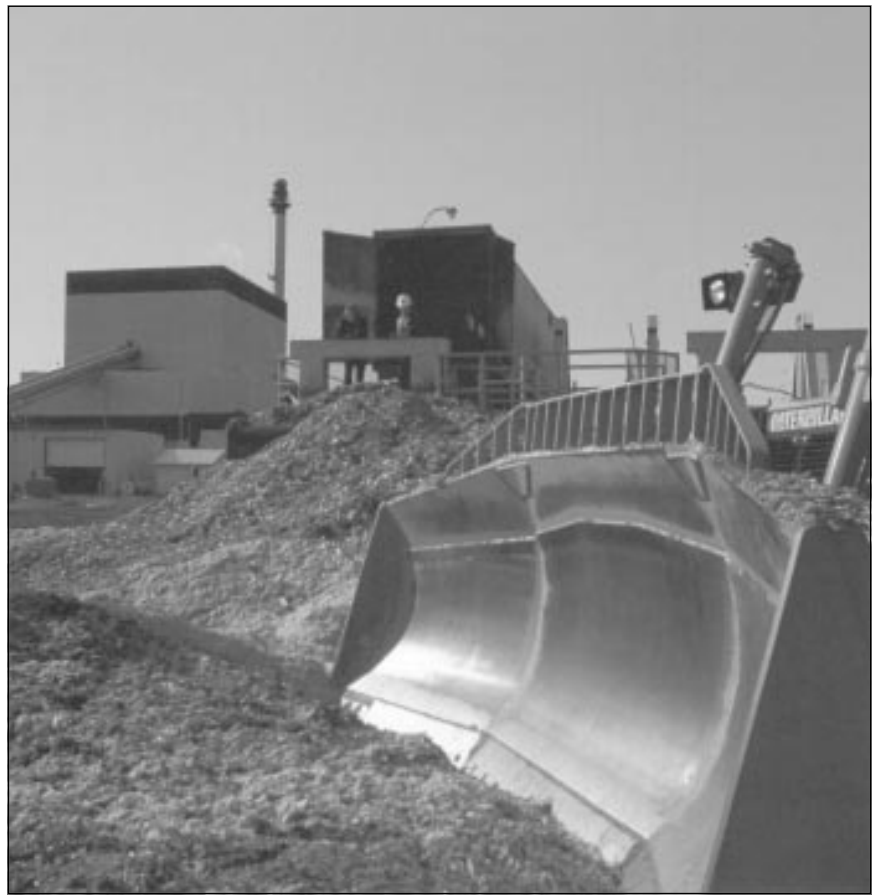
In energy farming, a two-to-three year cycle will yield up to 25 dry tonnes of timber per hectare per year. Burning chips create steam to run turbines. Energy-crop heat and power systems work well for midsize housing developments.
