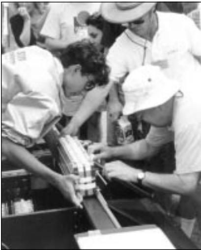
Once the vehicles left the road, the hard work began. Many teams had large, professional crews maintaining their vehicles. The Mitsubishi Materials Corporation team works on some silver zinc batteries, part of a 4.7 kWh storage bank.
