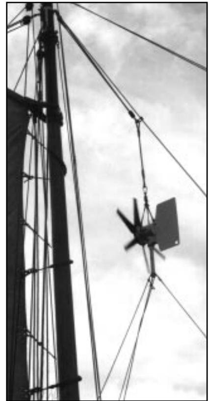
The Ampair hoisted into position hangs from the foresail sheet in the triangle between the mast and the forestay.
