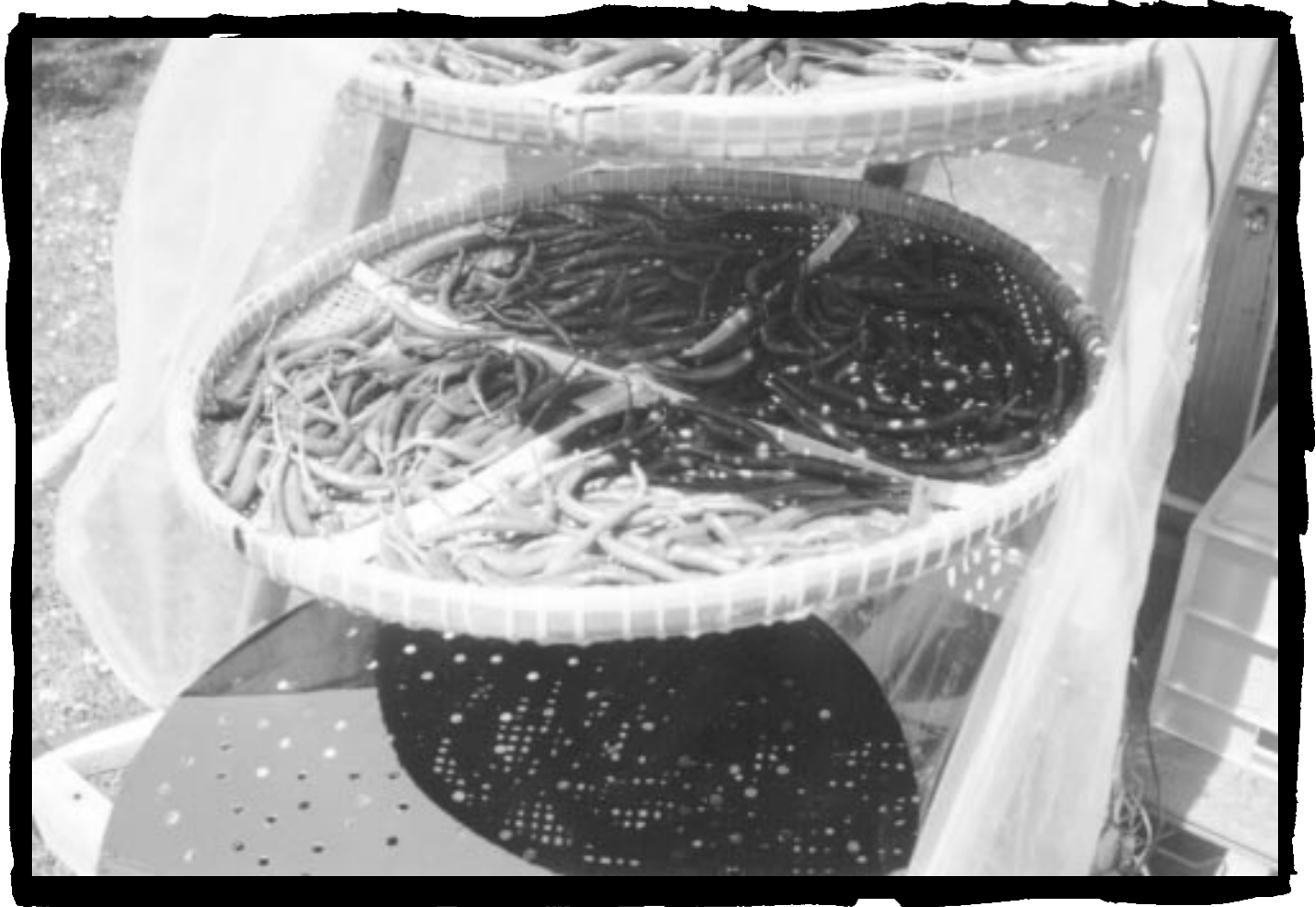
Over 50 kilograms of chillies were dried in the process of developing the drier, and tests included measuring the core temperature of the drying chillies on various trays.
