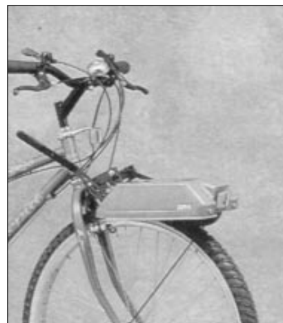
The Zeta can be fitted to almost any bike to provide power assistance.
