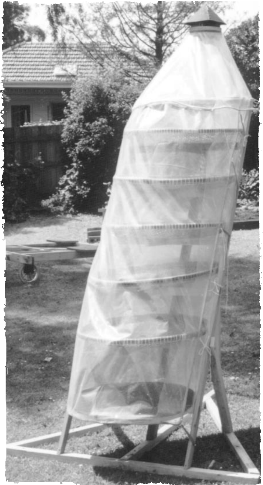
The fully assembled drier stands over six feet tall, and is capable of drying several kilograms of food at a time. Ian's drier is currently on display at the University of Melbourne International Development Technologies Centre.
