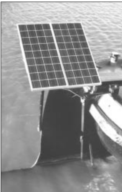
The Kyocera modules are mounted on the rudder post, keeping them out of the way of lines and activity on deck.
