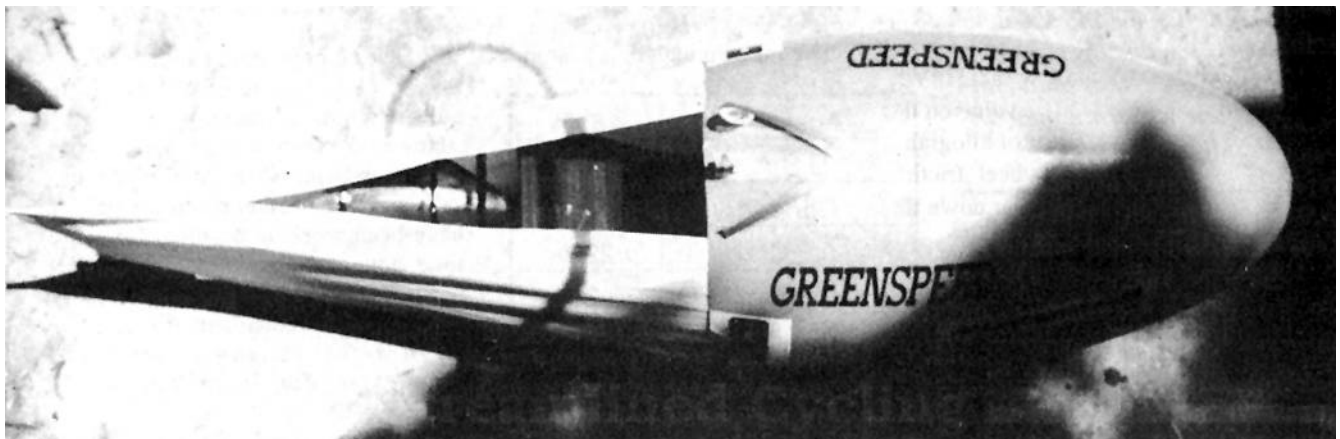
Figure 1. Bird's-eye view of the trike fairing, showing the tail shape and the little windscreen.
