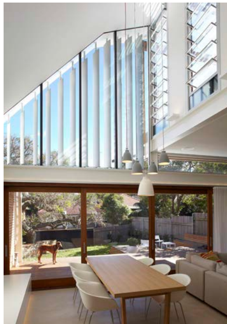
↑ Simon Anderson's Waverley house, showing the Fieger thermally broken low-e motorised louvres that are controlled by the home automation/climate control system.
