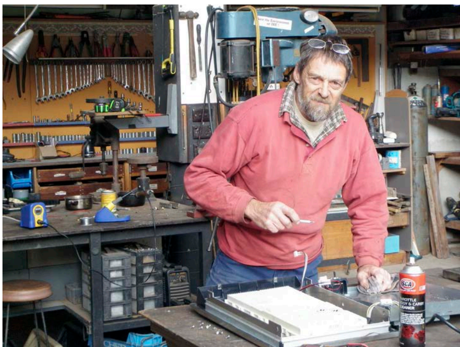
↑ John in his workshop, repairing a commercial induction cooktop. Two drops of vegetable oil on the control dial had rendered this unit (worth a few thousand dollars) almost worthless. A little degreaser and a clean rag soon fixed it. They now cook on solar-powered induction.
