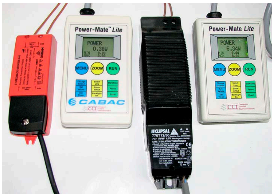
↑ Electronic transformers (at left) waste far less power than the old ferromagnetic ones while being smaller, lighter and producing less heat. Even with no load, the ferromagnetic transformer is wasting over five watts!
