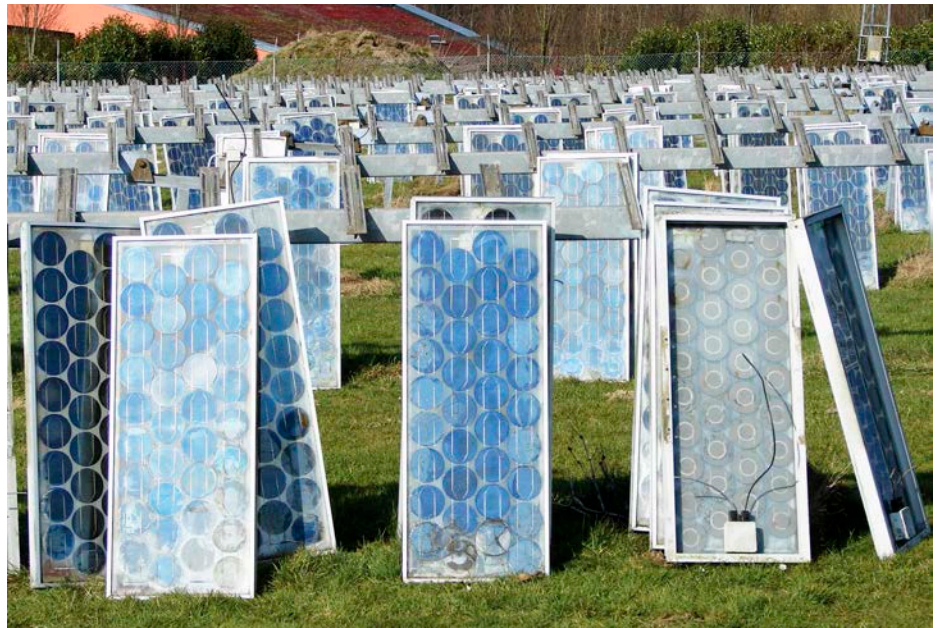
↑ Old PV panels contain large quantities of valuable materials such as aluminium, silver, tin and glass.
