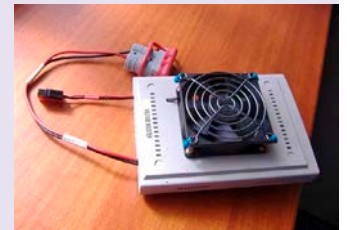
↑ The boost charger module, top, and the housing with fan.
