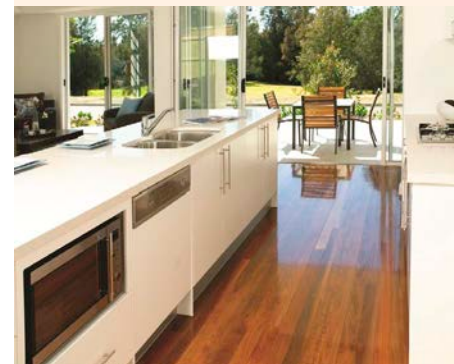
↑ To support ease of movement, a width of at least 1200 mm between kitchen benches is one of the 16 Livable Housing Design Guidelines.
