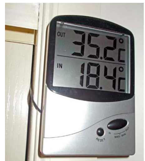
↑ The inside/outside thermometer has its outside probe located near the peak of the roof cavity.
