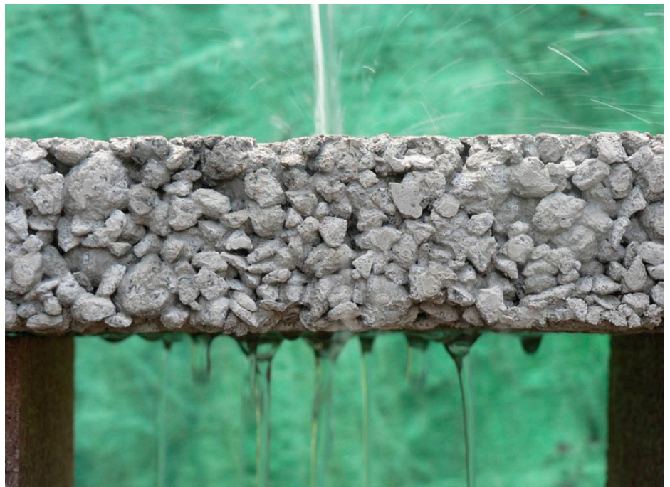
↑ Magnesium oxide based concretes not only capture CO 2 while hardening, they can be made into interesting materials such as this pervious concrete from TecEco, designed to reduce run-off from hard surfaces.
