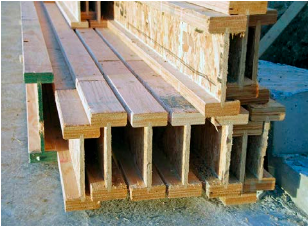
← Engineered timber, such as these Hyjoist beams, can provide high strength with much lower materials usage and weight.
