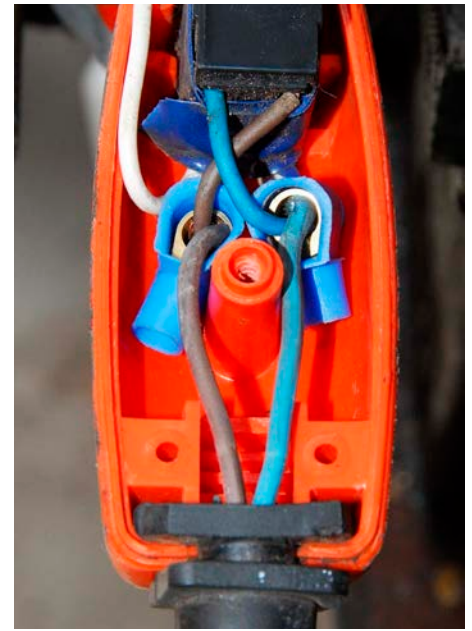
↑ With a couple of connectors you can fit a new cord.
