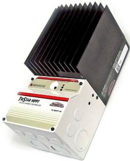
↑ DC coupled systems use a charge controller, such as this MorningStar TriStar unit. It features MPPT input up to 600V and full communications for system monitoring.
