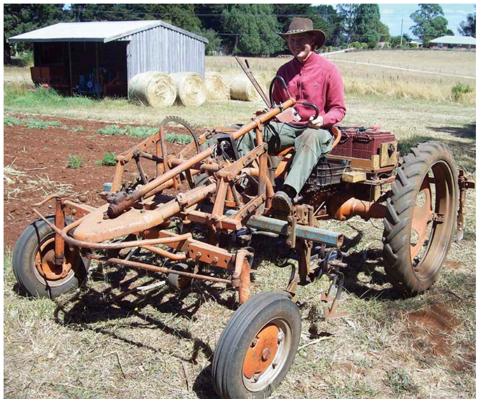
↑ The electric tractor—a conversion of an Allis Chalmers 'G'—is used for seeding and cultivating.
