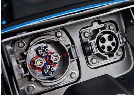
← The Nissan Leaf comes with two charging ports. A J1772 socket is on the right. The same plug is used for charging at levels 1 to 3. The socket on the left is the CHAdeMO.
