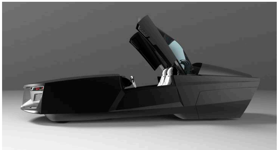
↑ A proposed design for Swinburne University's solar car, the Solaris. Surprisingly to many, one of the biggest challenges in car development is the sealing of doors. The clamshell design makes this a bit easier.
