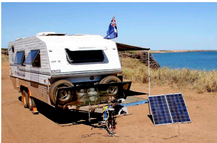
↑ Extra energy input can be gained by the use of additional folding solar panels—unfortunately, these are common targets for thieves in campgrounds and caravan parks.
