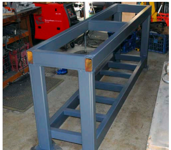
↑ The welded and painted frame. Note the number of cross-pieces used to give the lower shelf lots of support. You want to be able to place heavy items here to stabilise the bench.
