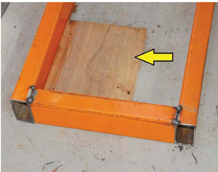
↑ The rectangular frame that underpins the benchtop was built first. Here it has been tack-welded and the shape is being checked for 'square' using the arrowed piece of board.
