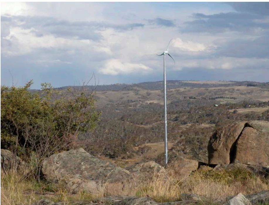
← This wind system appears to have great access to a wind resource, but it actually needs another 12 metres in height to get above turbulence created by the rough topography.
