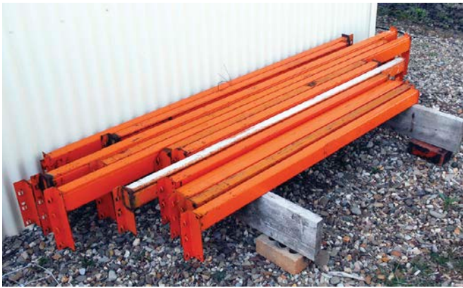
← These old pallet racking beams were cut and welded together to build the bench frame. Pallet racking beams in odd sizes and lengths are available very cheaply—these cost around $50.
