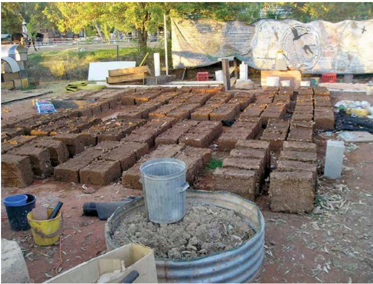
← Papercrete bricks being made.
