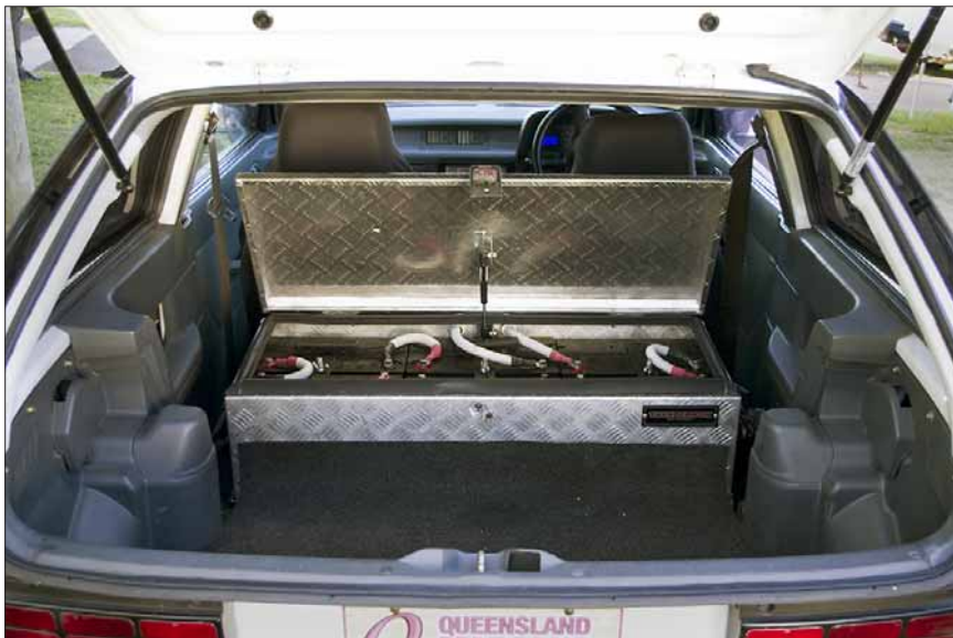
The main battery box replaces the rear seat.
