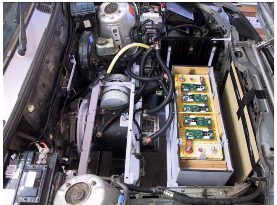
Inside the engine bay. Note the battery management units on the battery cells.
