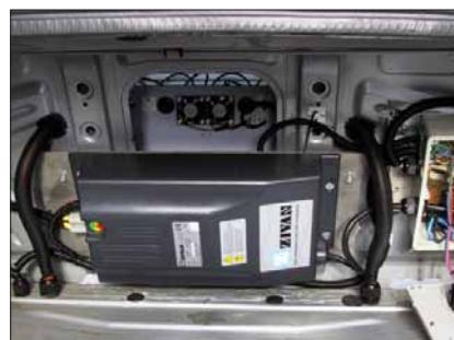
The Zivan battery charger lives in the boot, for charging on the go.
