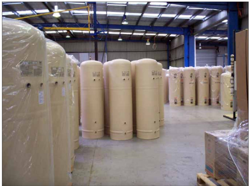
Everlast stainless steel tanks are one component of the solar hot water systems along with Solar Mio flatplate collectors, Grundfos pumps and Bosch boosters.
