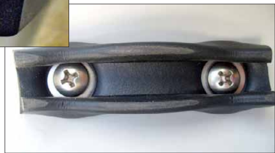
Pieces of U-channel foam are cut and punched and then bolted into the PVC half-section pipes. This prevents damage to the evacuated tubes when the cover is added or removed, or if it moves around in the wind.
