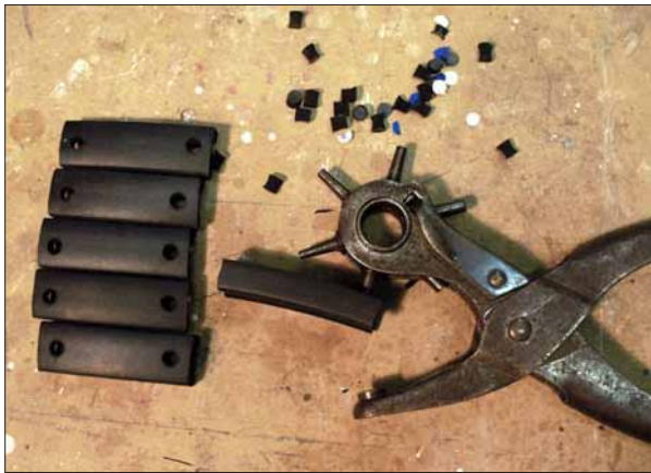
Pieces of U-channel foam are cut and punched and then bolted into the PVC half-section pipes. This prevents damage to the evacuated tubes when the cover is added or removed, or if it moves around in the wind.
