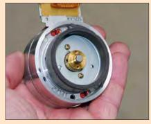
So what about that video drum again? Here's what a video drum assembly typically looks like. The first step is to undo all the visible screws...
