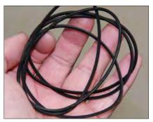
These belts (usually one per VCR) are also worth salvaging. I have used them as replacement belts in other machines but my major real-world use has been as gasket rubbers when I've wanted to seal around the top of a box or even inside the front of a bike headlight.
