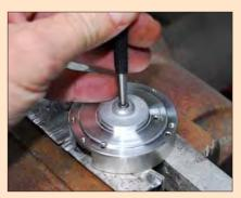
Some elements on the shaft are a press fit. However, the shaft is easily moved if the element is supported on vice jaws and a pin-punch and hammer are used to push the shaft through.
