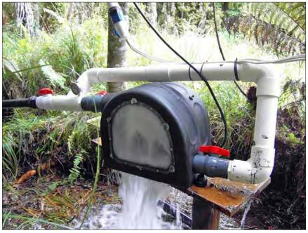
The new PowerSpout units from EcoInnovation use SmartDrive washing machine motors as very efficient generators.
