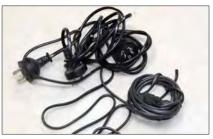
I also collect the power cords. These are invariably twin sheathed cable that's excellent when you want a reasonably heavy duty cable that looks neat and unobtrusive. For example, I've used this cable under the bonnet of cars to power accessories.
