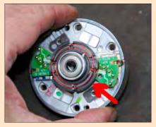
The parts like that arrowed here can be broken off with a screwdriver. Note that you should always wear goggles as this material easily shatters and is very sharp.
