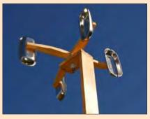
Amongst other things, I've used video drum assemblies to make wind vanes and manual anemometers. To assess wind speed you just watch how fast it is turning—the precision bearings make it incredibly sensitive.
