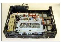
It takes very little time to remove the cover (keep those screws!) and strip out the main circuit boards. In fact, it's worth stressing that disassembling a VCR is really a quick and easy process. Expect to take perhaps only half an hour to do the first one from start to finish. When you get speedy, you can do it in 10 minutes.
