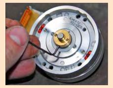
The brass collar is held in place on the shaft with an internal Allen head grub screw. You'll need the right sized Allen key—don't try to drill out the grub screw as the (working) collar is very valuable.
