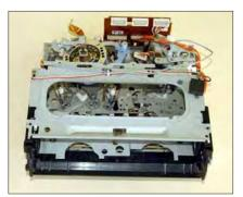
Here's the inner chassis on its own. As you can see, already the contents of the VCR have been narrowed down to just this and the electronic circuit boards.
