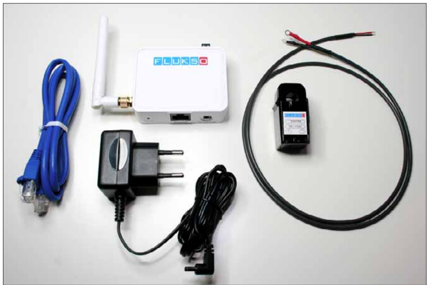
The kit, clockwise from bottom: power supply, cables, Fluksometer wifi device and current sensor.
