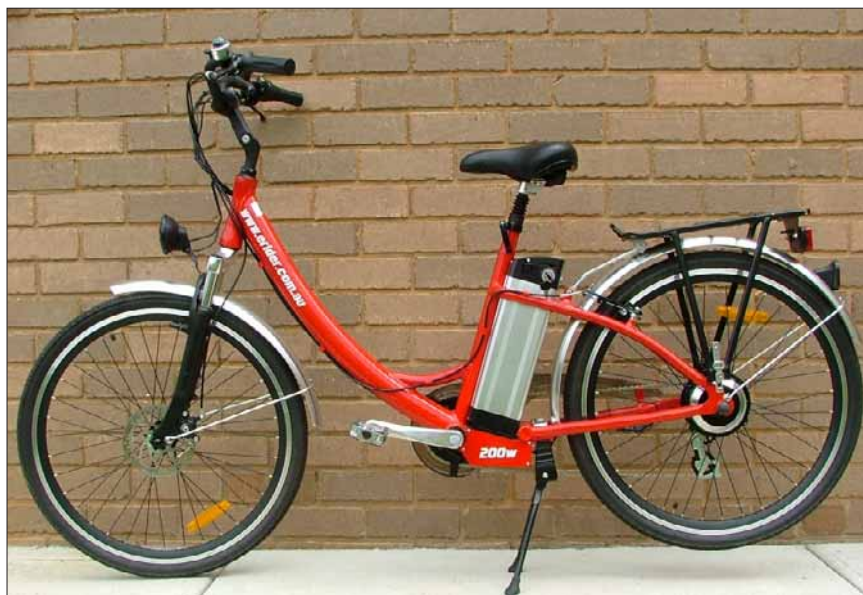
A typical electric bike. This one is from Erider Electric Bicycles. Note the battery pack behind the seat post and the hub motor in the wheel—a common configuration.
