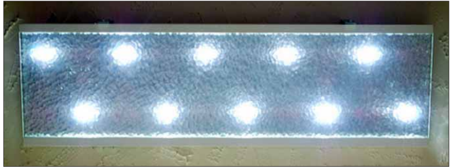
The finished skylight. You can clearly see the 10 LEDs, wired as two strings of five.
