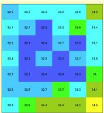
These 'thermographs' were taken of the ceilings of four different rooms (the kitchen, bedroom, living room and bathroom, clockwise from top-left) inside the same home by measuring the ceiling temperature at regular spacings. The temperature ranges were then assigned a colour for easy visualisation of temperature variations.
