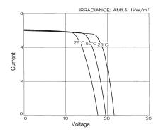
Figure 1. These IV (current-voltage) curves for a typical 80 watt polycrystalline panel show how power output is affected by temperature. You should take this into account when buying panels.
