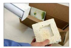
The material is resistant to mould and mildew, uses very little energy to manufacture and can simply be composted at the end of its useful life. Ecocradle can be made into any shape to suit whatever product it is protecting, just like styrofoam.
