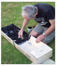
Top: It all starts with a couple of boxes from the supermarket. Note the collector box has been taped together. Right: Lindsey preparing the collector box with black paint. Bottom: Making the top transition.
