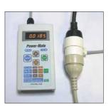
measuring via a simple piggyback plug and socket set. The meter features an LED display for easy reading and high visibility at all times.
