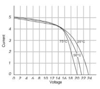
Figure 2. The IV curves for a 64 watt amorphous panel. Note how the maximum power point at the knee of the curves barely moves with increasing temperature.
