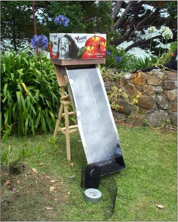
Top: The kids have abandoned the project while the adults work out the next step with the collector box. Left: The apple box with the mesh ready to be pushed in. Above: The completed solar dryer, made from cardboard boxes, a single sheet of glass, chicken wire and plenty of black paint.
