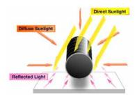
The novel Solyndra panels use glass tubes lined with thin film material rather than flat sheets of glass like regular panels.
