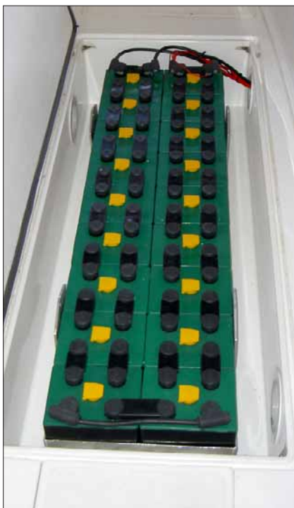
There's no fuel tank of course, just a bank of 18 batteries hidden away under a seat.
