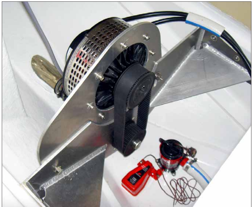
The high-efficiency electric motor is tiny compared to most boat motors.
