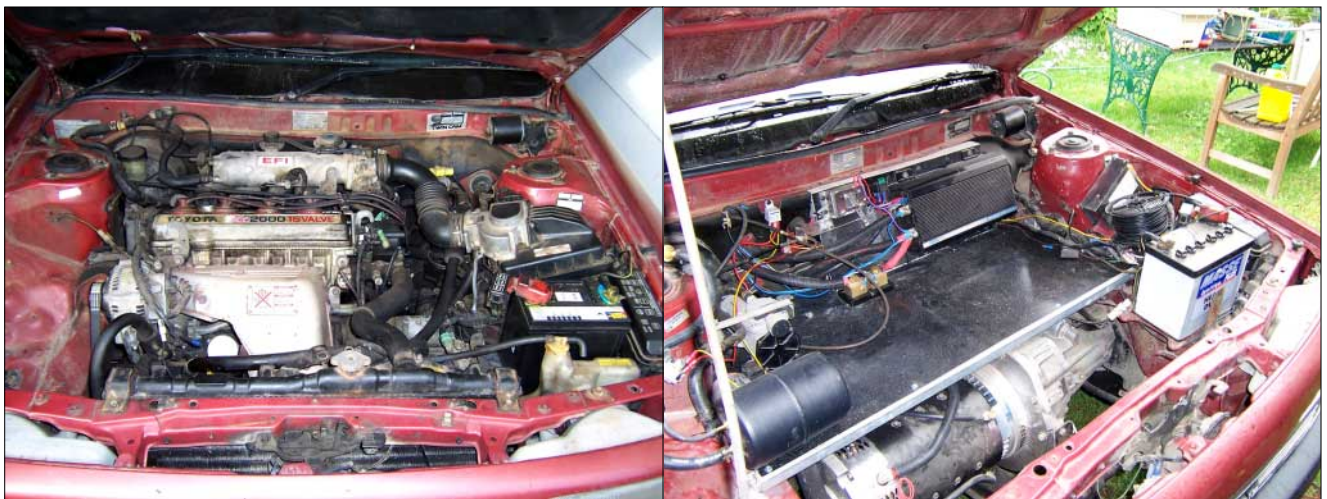
Out with the old, in with the new. Before and after shots of a typical EV engine bay. As you can see, the electric system is a lot simpler than the petrol one!
