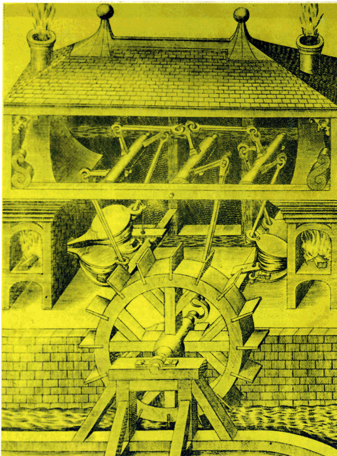
Furnace with water-driven bellows, 16th century.
