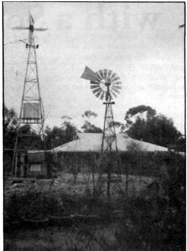
The secondhand 32 volt Dunlite windgenerator and windpump standing near the house.
