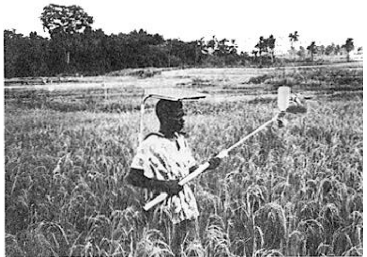
Panel of solar cells acts as sunshade and also powers an insecticide sprayer.
